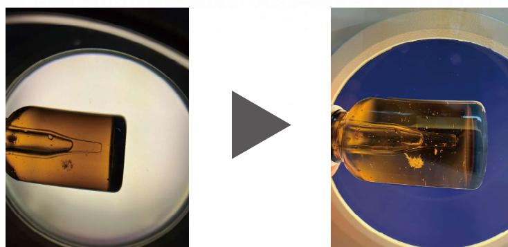
By adjusting the rotating frame, foreign particles inside the container become visible.
